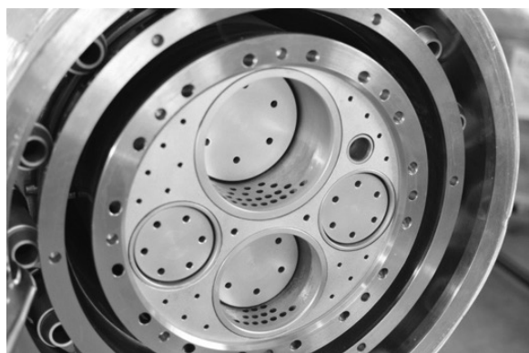
Figure 2. Unitherm Cemcon's dynamic M.A.S. kiln burner with two integrated solid secondary fuel channels equipped with the patented PNEUMO-DEFLECTOR nozzles.
